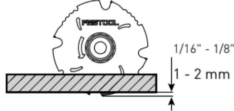
Set the cutting depth according to the workpiece thickness – tooth projection of  $1/16" - 1/8"$  (1-2 mm).
